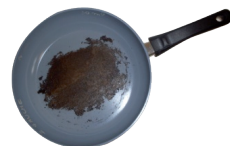
Ceramic frying pan after 1,000 abrasion cycles
