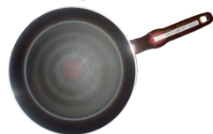
T-FAL New Intensium frying pan after 16,000 abrasion cycles
